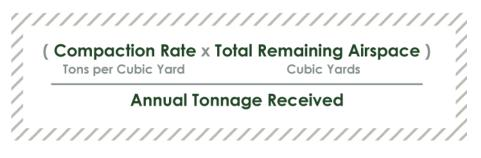
As of 2020, Rumpke has been compacting waste at a higher rate. Packing more waste into each cubic yard of airspace will affect the projected remaining useful life of the landfill. Rumpke is also reporting waste receipts of around 1,000 tons per day, which also affects remaining useful life projections.
